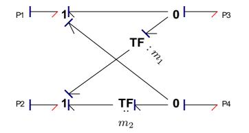
With an all-input power convention,  $(e_1, e_2, f_3, f_4)$  would be obtained from  $(f_1, f_2, e_3, e_4)$  with an antisymmetric matrix. With the through-power convention, the matrix is symmetric and can be decomposed into two matrices wich are transpose:
