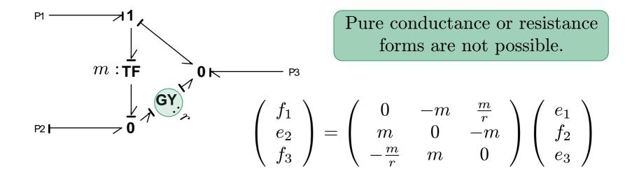
Multiport transformers are an special case of junction structures.
