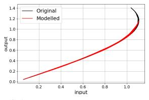
Fig. 3. Generic comparison between desired inverse function and modeled response.
