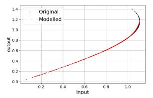
Fig. 5.Memoryless inverse response without one-to-one mapping.
