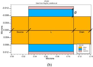
Fig.1. Schematic view of a Cylindrical Vertical device (a) and its schematic representation of the cross section along the channel A-A'(b).
