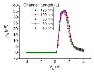
Fig. 3. Transconductance  $(g_m)$  as a function of channel length (L) for  $V_D = 500 mV$ .
