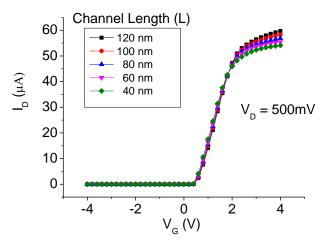
Fig .2.  $I_D x V_G curves$  for different channel lengths.
