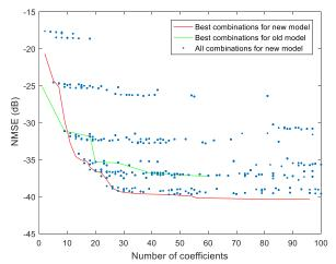
Fig. 2. NMSE values as a function of the number of coefficients for the LTE band.
