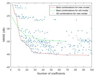
Fig. 1. NMSE values as a function of the number of coefficients for the WiFi band.
