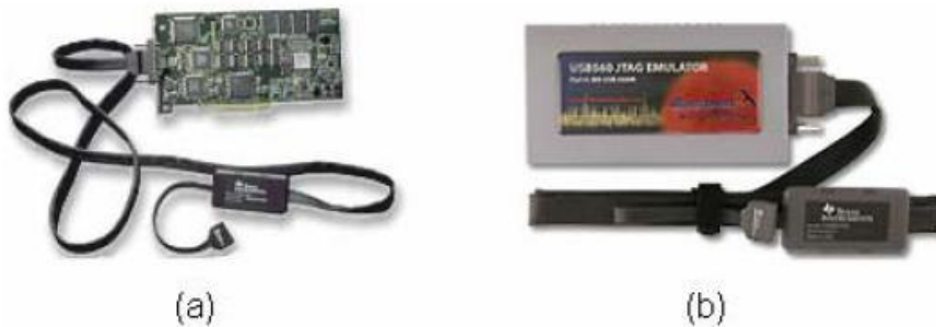
Figura 3 – exemplo de emuladores JTAG. (A) XDS560 PCI-BUSS JTAG SCAN_BASED EMULATOR (DSP8032U). (B) BLACKHAWK XDS560 USB EMULATOR (DSP11990U)
